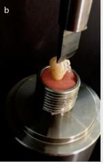
**Figure 1.** (a) Application of the solvents, (b) Shear force applied with the Universal Test Machine.
