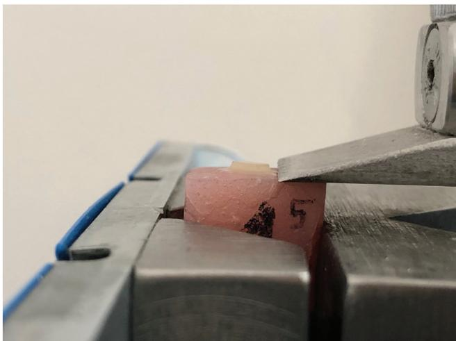
**Figure 1.** The SBS test
