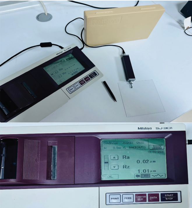
Figure 2. Surface roughness measurement using Surftest SJ-301 (Mitutoyo, Kanagawa, Japan).
